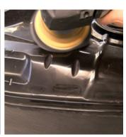
Moulds made using Uni-Mould are highly polishable to a full gloss and can easily be restored if they are subject to light scratches using a composites polishing compound (such as Mirka T10). After polishing, ensure a thorough re-application of release agent before use.
