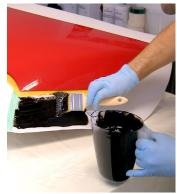
Uni-Mould Tooling Gel Coat should be catalysed at 1.5-2% using standard MEKP catalyst. Before application allow the catalysed gel coat to stand for a few minutes to settle and de-gas.
