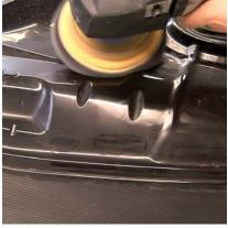
Moulds made using Uni-Mould are highly polishable to a full gloss and can easily be restored if they are subject to light scratches using a composites polishing compound (such as Mirka T10). After polishing, ensure a thorough re-application of release agent before use.
