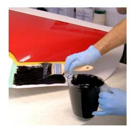
Uni-Mould Tooling Gel Coat should be catalysed at 1.5-2% using standard MEKP catalyst. Before application allow the catalysed gel coat to stand for a few minutes to settle and degas.
