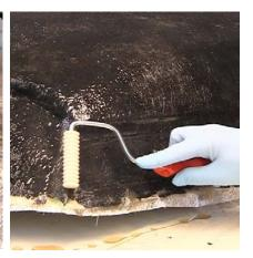
The Uni-Mould Coupling Coat is designed to eliminate print-through of the mould reinforcement, to reduce the risk of blisters underneath the gel coat by ensuring the gel is reinforced with a skin of resin and glass and to provide an ideal substrate for the main reinforcement.
