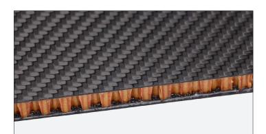
Nomex® honeycomb carbon fibre panel made using XC130 prepreg and XA120 adhesive film.
