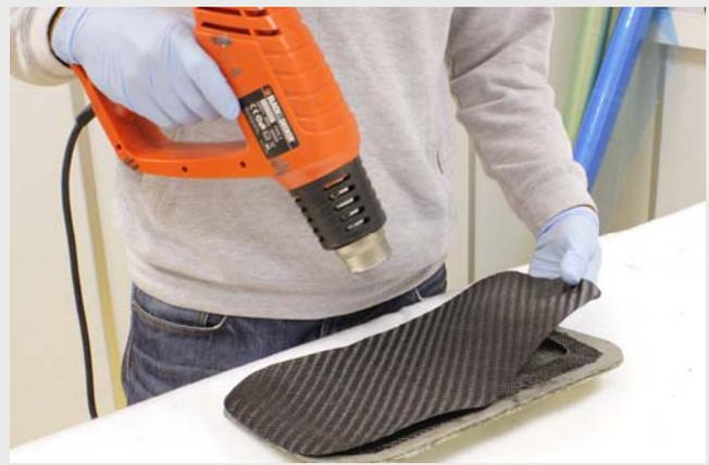
Gentle use of a heat gun is recommended on the backing ply/plies to make the prepreg softer and more drapable.
