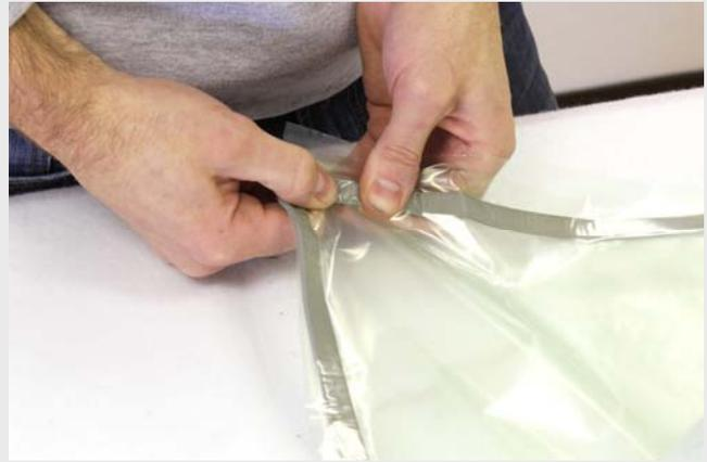
At this stage, seal 3 of the 4 edges. Press and squeeze the bagging tape very firmly to ensure an airtight seal.
