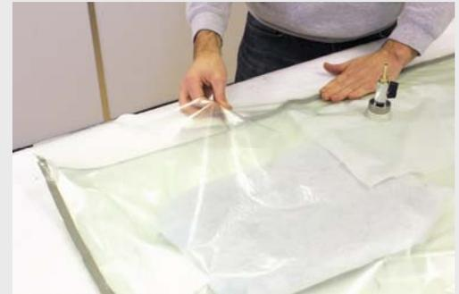
Tape-up the last open side of the bag and press and squeeze the seal firmly.
