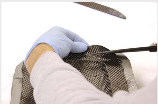
Once down, trim off any excess material so that the prepreg does not reach the edge of the mould's flange.
