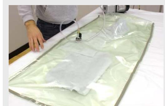
An 'envelope bag' completely encloses the part(s) instead of bagging film being pleated and taped to the mould's flange.
