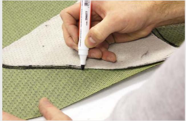
The backing ply can easily be marked using a permanent marker pen on the removable film.
