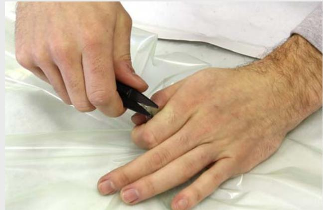
Snip off the top 5mm of the peak to make a circular hole in the film of about 12mm.
