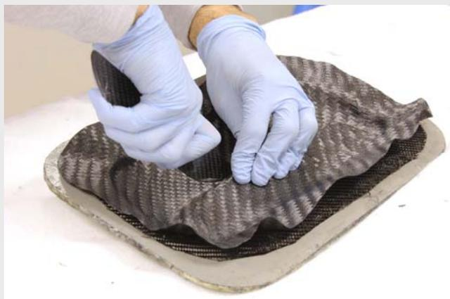
Just like with the surface ply, blunt tools are recommended to press the prepreg firmly into any tight corners of the mould.
