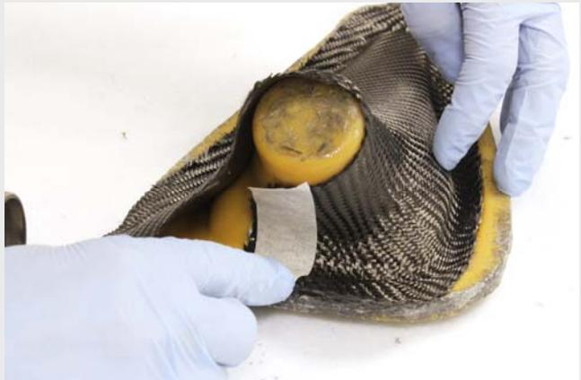
To create a perfectly straight seam at the back of the duct where the material meets, masking tape is used to mark a vertical line.
