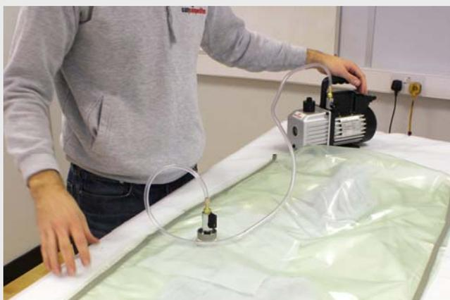
Connect the pump to the through bag connector using a length of silicone or PVC hose. Remember that silicone hose must be used on the part in the oven.
