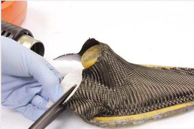
The surface ply can then be gently peeled away from the mould and cut perfectly along the tape line.
