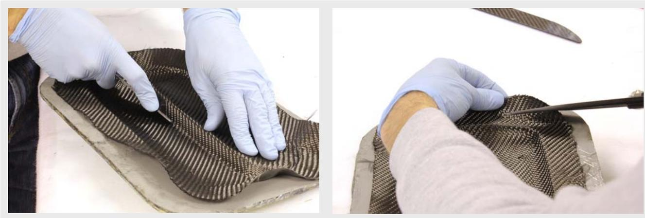
Remember, just like with the surfacing layer it is essential that the backing layer or layers are firmly pressed down into all areas of the mould, especially tight or awkward corners. Take lots of time doing this as it will make all the difference between a perfect part and a failure.
