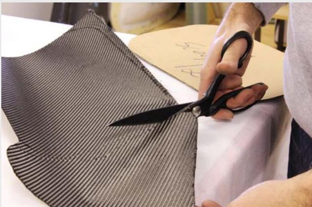
The Easy-Preg surfacing ply is easily cut with a pair of composites shears or normal scissors.
