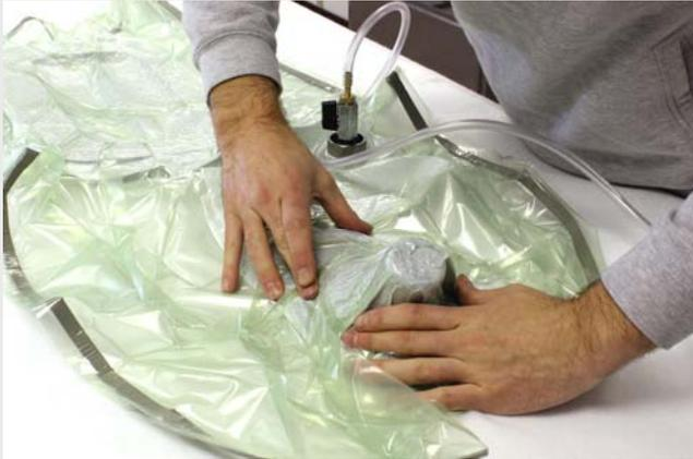
Push plenty of 'wrinkles' of bag into difficult shapes like the underside of this duct. The more wrinkles the better!
