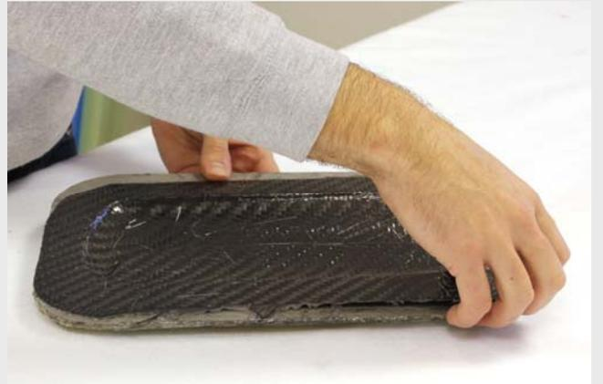
Releasing parts is simply a matter of sliding a fingernail or plastic card under an edge of the cured laminate.
