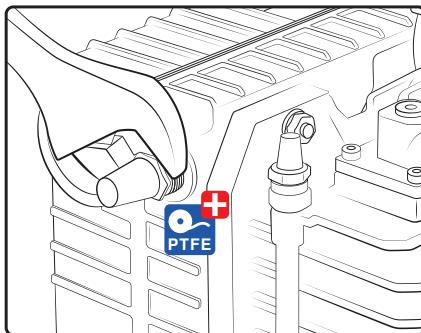
Using a spanner, screw the exhaust silencer into the outlet on the **LC20EC** vacuum pump.
