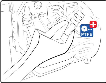
Tightly screw the 90° brass elbow fitting into the 1/2" port on the *LC20EC* vacuum pump. Finish with the fitting facing upwards.
