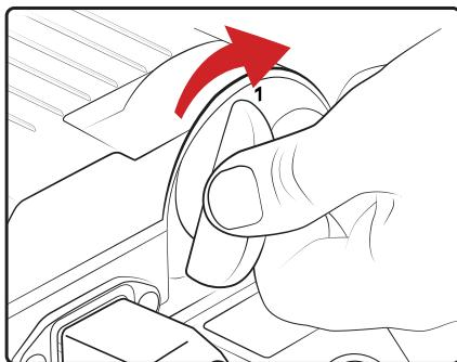
Switch off the pump to stop the degassing process.
