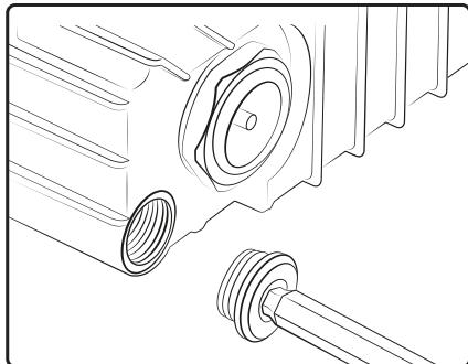
If the oil appears cloudy, discoloured or contaminated at any time, drain the old oil from the vacuum pump using the drain screw and then refill the pump with fresh vacuum pump oil.
