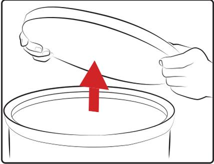
Start by removing the acrylic lid and loading your material (casting resin, RTV silicone rubber etc.) into the degassing chamber.
