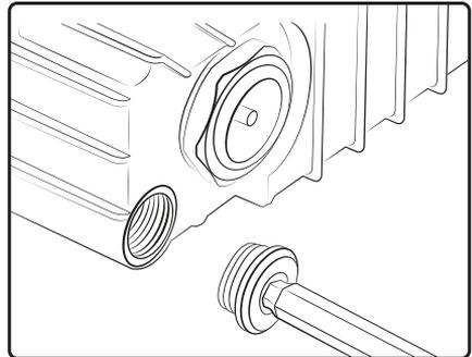
If the oil appears cloudy, discoloured or contaminated at any time, drain the old oil from the vacuum pump using the drain screw and then refill the pump with fresh vacuum pump oil.
