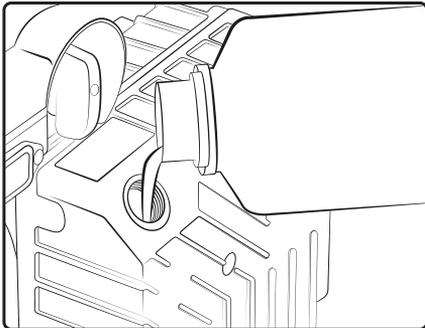
Unlike conventional oil-bath vacuum pumps, the **LC20EC** emits virtually no oil from the pump during operation however, depending on how frequently you use your vacuum pump and how you are using it, you still need to periodically check and top-up the oil level to ensure it stays at the recommended level.
