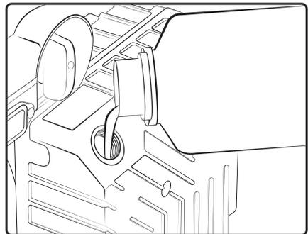
The *LC20EC* pump ships without oil and needs to be filled to the correct level using the supplied oil before use.
