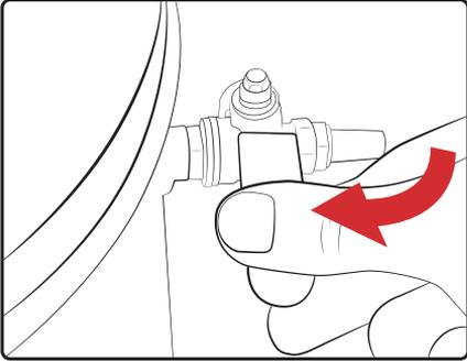
Make sure the inlet valve (which has the brass filter fitted) is in the closed position, especially if you have just run a degassing operation.
