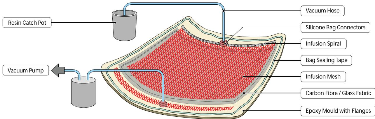
There are many alternative configurations to the above that can be used for resin infusion. The above configuration, however, is quite typical and makes a good starting point.
